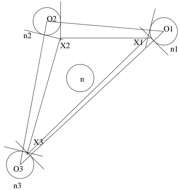
Fig. 2. Node  $n$  in the interior triangle of three trusted nodes
